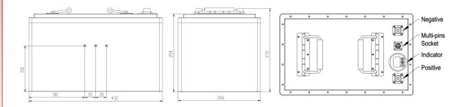
Here is a multi-pins socket built on the top of battery pack,
